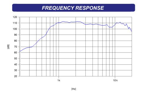
Note: On axis frequency response measured coupled to TD-385 horn in anechoic chamber, 2,83 v @ 1m
